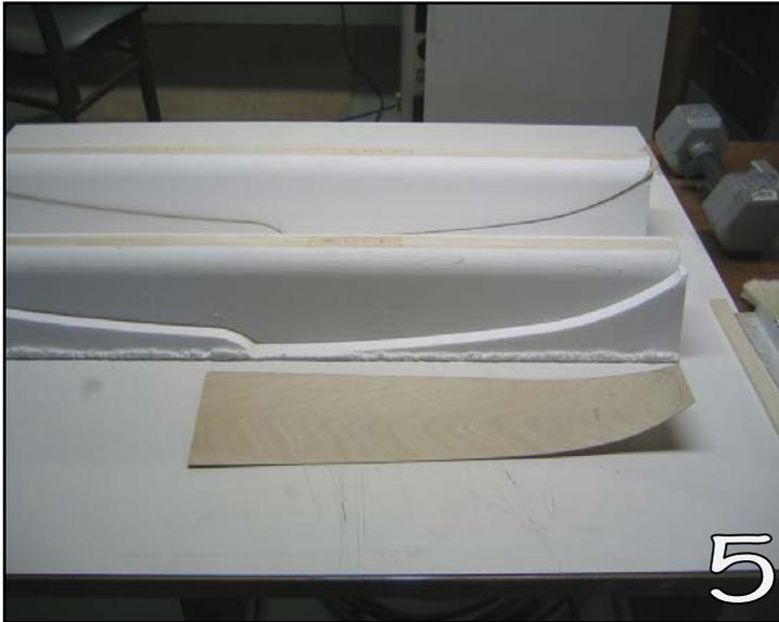
Make a template for the shape of the bottom front and cut the 1/32" aircraft plywood to shape. Soak the front of the plywood in warm water for a few minutes and then place between the float and the bottom form to dry. When dry it will be curved as in above photo and is very easy to attach using the Sorghum. Sand the front plywood edges flush with the foam sides and round the tip to conform to the shape of the foam.
